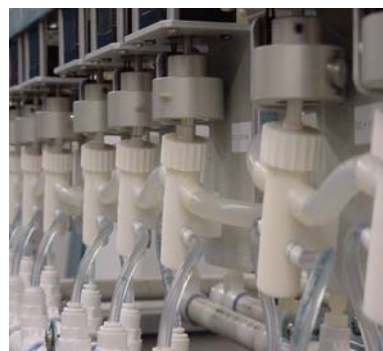
Piston pumps undergoing long-term life testing
